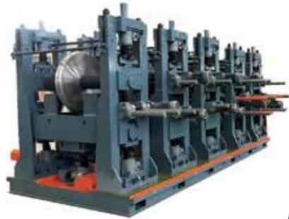
1. Can produce straight welded round, square, rectangular, and unwelded abroach steel(C,Z,U,etc) within **1 set of production line.**
